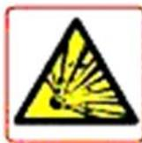
***Explosion warnings-*** The explosion warning symbol is an explosion mark enclosed in a triangle. The Explosion warning symbol is used to indicate locations and conditions where molten, exploding parts may cause serious injury or death if the proper precautions are not observed
