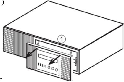
2. ONLY IF NECESSARY, cut the left-hand Zip Tie to access the retaining screw
