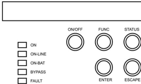
**Figure 4 Control panel – 2400VA Tower/6000VA Rack Unit**
