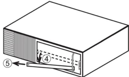
6. Pull Battery Tray out of UPS chassis.
