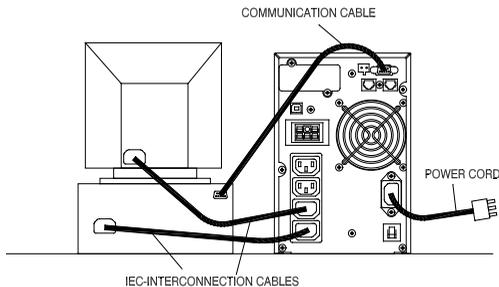
**Figure 2 Example of Installation of Plug & Play products.**
