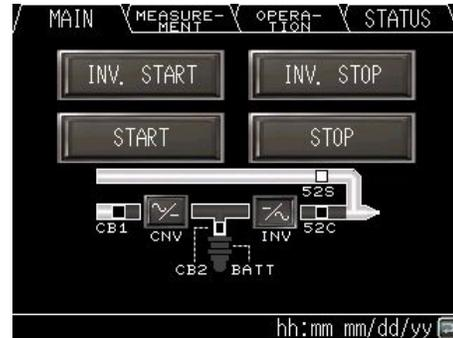
Figure 4-3 Startup/Shutdown Guidance
