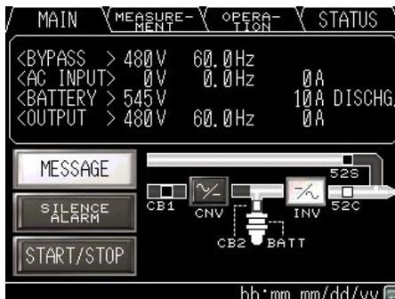
Figure 4-14 Main screen (Fault indication)
