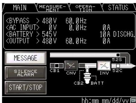
Figure 4-12 Main Screen (Battery Operation)
