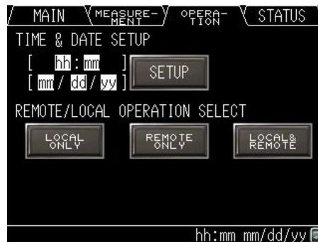
Figure 4-8 Remote/Local operation and Date & Time adjustment select
