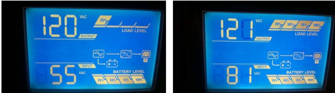
We recently did some testing of small UPS. These were the Orion Online RT, the Orion Office Pro and the APC SmartUPS. We varied input voltage to each UPS to test voltage regulation in normal operation and to determine when they transfer to battery.
