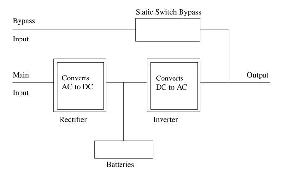
The selection of components in the rectifier and the inverter affects input characteristics, output characteristics as well as battery and bypass use. The goal is to satisfy output demands of the supported critical load while minimizing use of batteries and bypass and to minimize problems created by the input. Stating that is the simple part.
