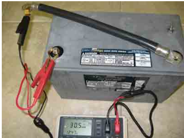
12.47 VDC, 30.5 m-ohm, bolt missing
