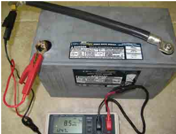
12.47 VDC, 8.5 m-ohm, bolt in place
